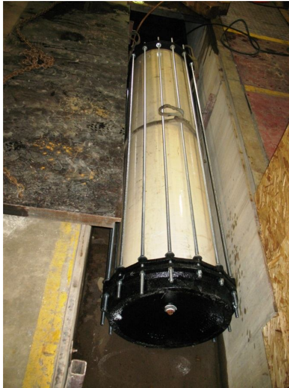
Figure 1. Photo of sample #3 prior to structural integrity testing.
